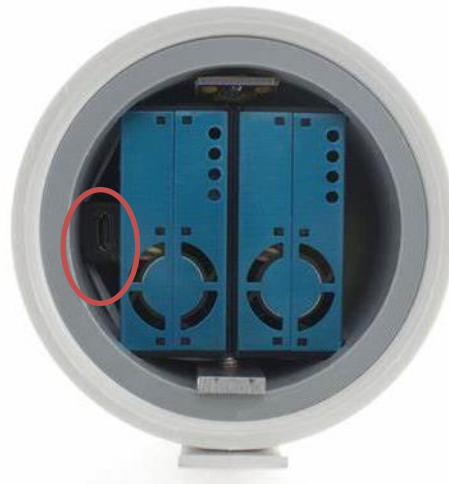
Figure 5. The bottom part of the PurpleAir sensor. The light that turns on when the sensor is in operation is marked with red circle.
